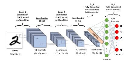
Stacking multiple layers of conv network will decrease the overall dimensionality. Finally, we can flatten the 3-d tensor to a 1-d vector, which is used to do classification.
