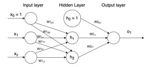
$\rightarrow$  Hint: Start by converting XOR to logical formula composed of logical operations that can be represented by a perceptron:  $o_1 = (x_1 \lor x_2) \land (\neg(x_1 \land x_2)) = h_1 \land h_2$
